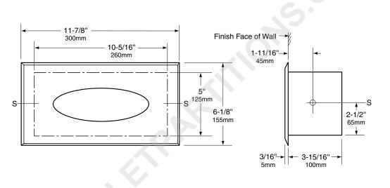
Rough Wall Opening 10-3/4" (275mm) wide 5-1/4" (135mm) high 4" (102mm) minimum recessed depth
