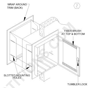
MOUNT AND ADJUST WRAP AROUND BACK TRIM TO WALL THICKNESS
