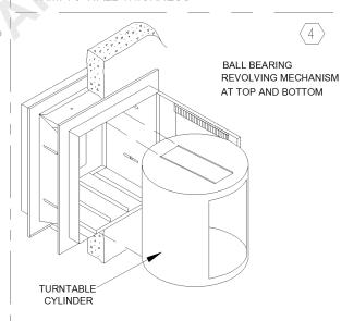
INSERT CYLINDER INTO CORRESPONDING TRACKS AT TOP & BOTTOM OF BOX. CLOSE & LOCK DOOR.
