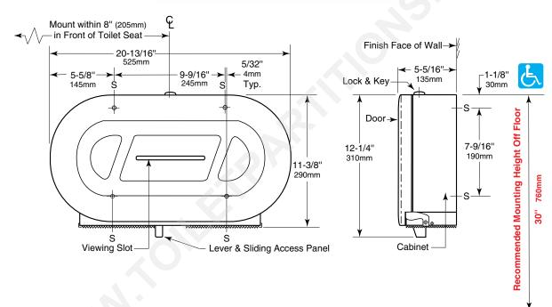
**Note:** Dispenser is ICC A117.1 - 2009 Standard for Accessibility compliant. Unit can be located below grab bar, in area 24" minimum to 42" maximum from rear wall, with outlet 18" minimum above floor.
