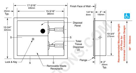
Rough Wall Opening 15-5/8" (395mm) wide 11-1/4" (285mm) high 4" (100mm) minimum recessed depth
