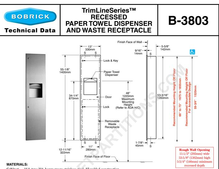
Cabinet — 18-8, type-304, heavy-gauge stainless steel. All-welded construction.
