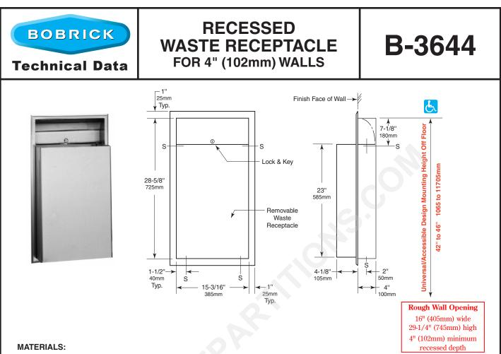
Cabinet — 18-8, type-304, heavy-gauge stainless steel. All-welded construction. Exposed surfaces have satin-finish.
