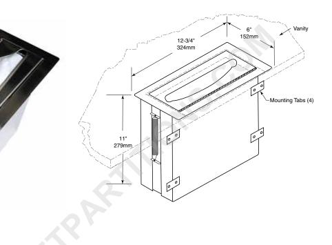
Rough Countertop Cutout 11-1/4" (286mm) Wide 4-1/2" (114mm) High 3/4" to 1-1/2" (19 to 38mm) mounting thickness 17" (430 mm) minimum clearance below mounting surface
