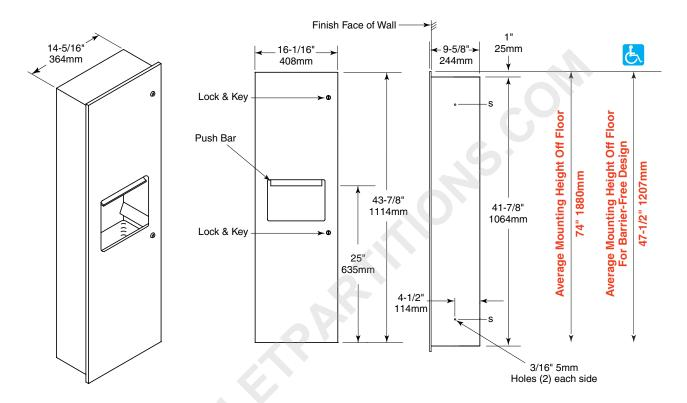
Rough Wall Opening 14-5/8" (371mm) Wide 42-3/8" (1073mm) High 9" (229mm) minimum recessed depth
