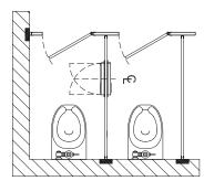
5900 Series Combination Units are to be installed so that doors open 90° to fill product and maintain waste container.
