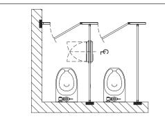
5900 Series Combination Units are to be installed so that doors open 90° to fill product and maintain waste container.
