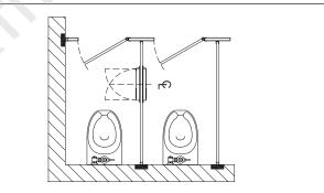
5900 Series Combination Units are to be installed so that doors open  $90^\circ$  to fill product maintain waste container.
