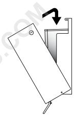
1. Mount dispenser to wall using enclosed screws and wall plugs.
