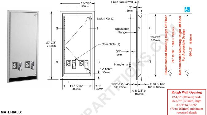
Cabinet — 18-8, type-304, 22-gauge (0.8mm) stainless steel. All-welded construction.
