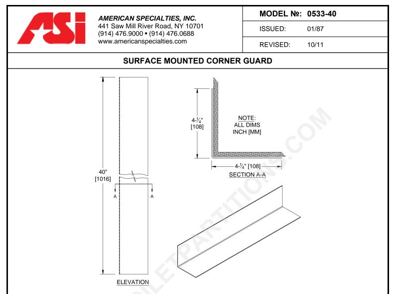
Surface Mounted Outside Corner Guard shall be 18 gauge type 304 alloy 18-8 stainless steel with a 1/8" (3.2) radius outside edge. Width of guard on each side shall be 4-1/4" (108) x 40" long (1016). All exposed edges shall be smooth and fully debarred. Back surface shall be rough textured to facilitate adherence to wall surface. All exposed surfaces shall be satin finish and be protected during shipment with a PVC film easily removable after installation.
