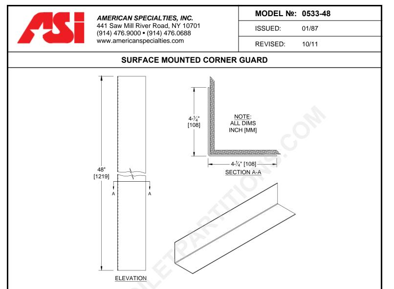
Surface Mounted Outside Corner Guard shall be 18 gauge type 304 alloy 18-8 stainless steel with a 1/8" (3.2) radius outside edge. Width of guard on each side shall be 4-1/4" (108) x 48" long (1219). All exposed edges shall be smooth and fully debarred. Back surface shall be rough textured to facilitate adherence to wall surface. All exposed surfaces shall be satin finish and be protected during shipment with a PVC film easily removable after installation.
