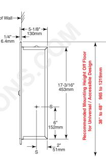
Rough Wall Opening 12" (305mm) wide 17-3/8" (441mm) high 5" (127mm) minimum recessed depth
