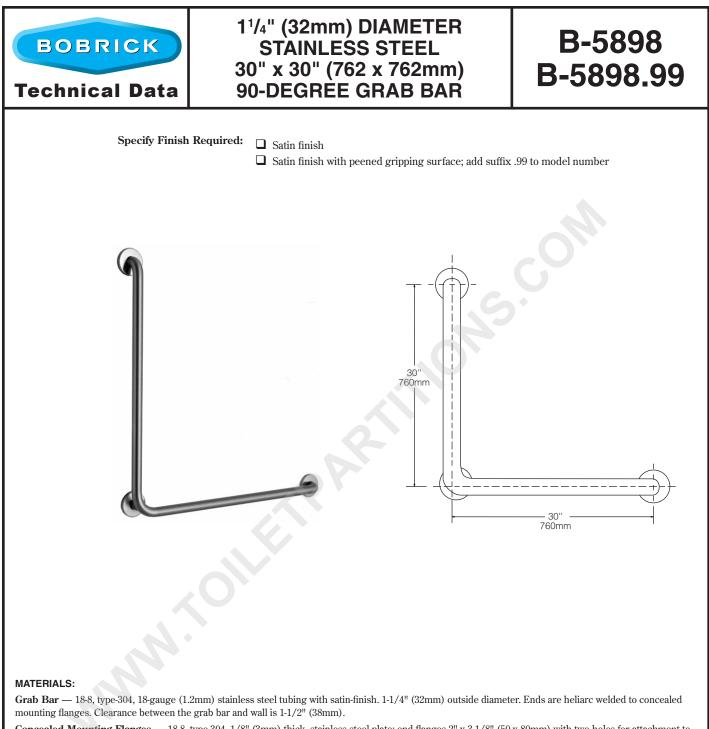
**Concealed Mounting Flanges** — 18-8, type-304, 1/8" (3mm) thick, stainless steel plate; end flanges 2" x 3-1/8" (50 x 80mm) with two holes for attachment to wall. Intermediate flanges 2-5/8" x 3-1/8" (65 x 80mm) wide x 3-1/8" (80mm) diameter.
