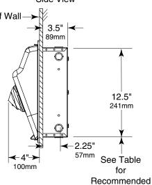
Recessed Mounted Unit with ADA Compliant Q Nozzle
