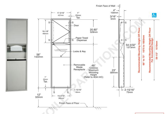
Rough Wall Opening 16" (406mm) wide 54-3/4" (1390mm) high 4" (100mm) minimum recessed depth
