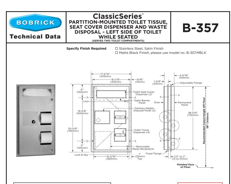
**Note:** For accessible toilet compartments, please use horizontal recessed or surface -mounted combination dispenser-/disposal-units, B-3091 or B-3092 Series, to comply with ADA 1-1/2" absolute Grab Bar wall spacing.
